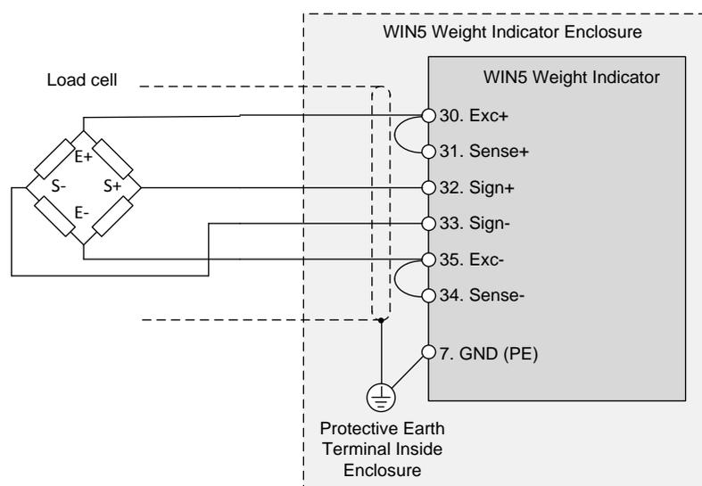
Figure 2.12 Connection of Load cell without Junction Box.
