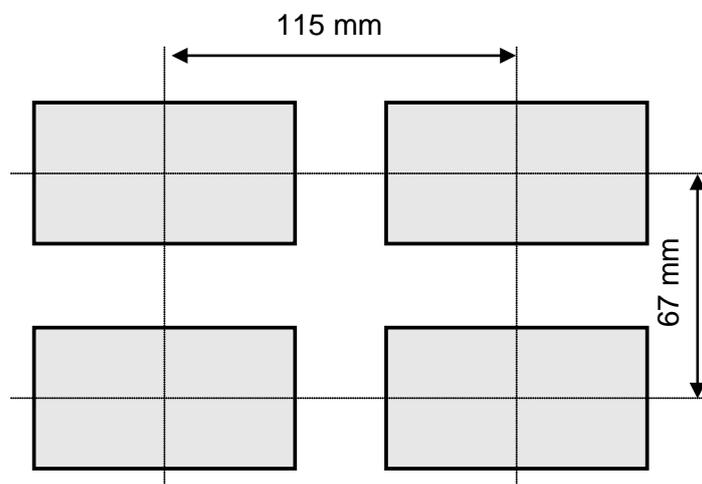
Figure 2.4 Minimum distances when assembly of a number of units
