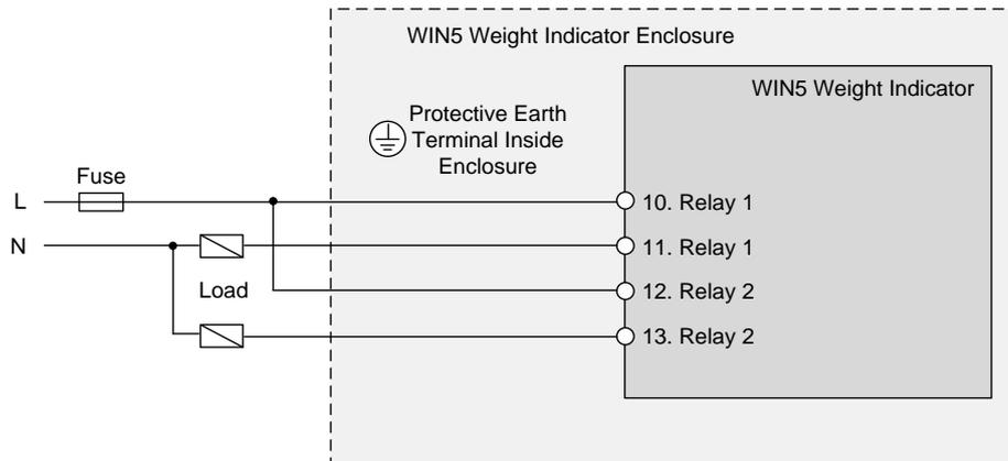
Figure 2.6 Connection of Relay Outputs, PE wires should be connected to the PE Terminal inside the enclosure.
