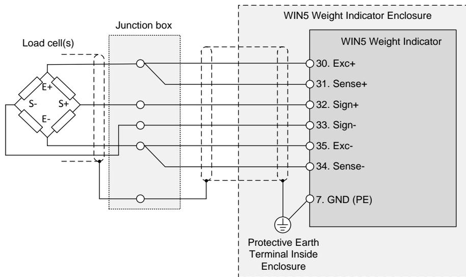
Figure 2.11 Connection of Load cell(s) with Junction Box.
