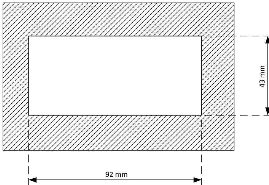
Figure 2.2 Allowable mounting hole dimensions
