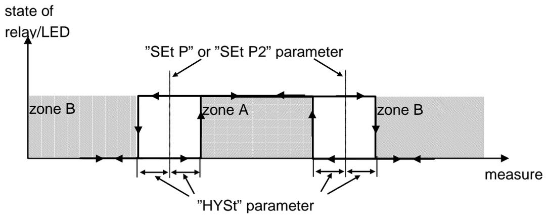
Figure 4.3 Two threshold control of the relay/LED outputs
