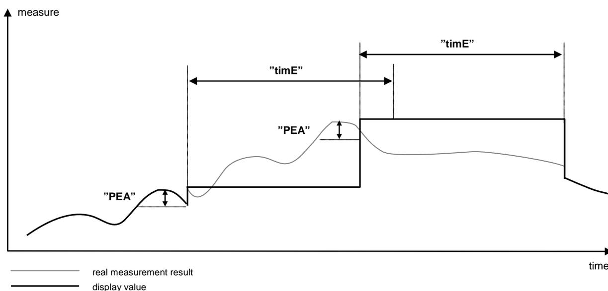
Figure 4.1 Process of peaks detection
