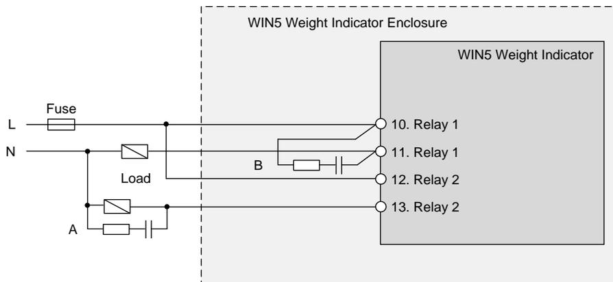
Figure 2.7 Examples of suppression circuit connection:
