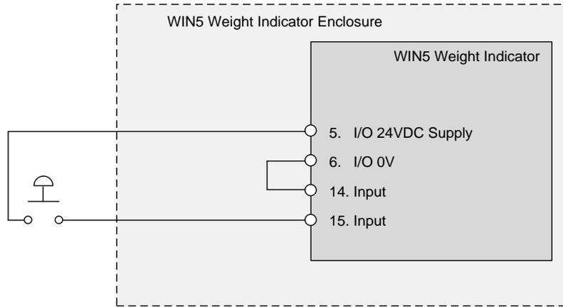
Figure 2.8 Connection of Digital Input.
