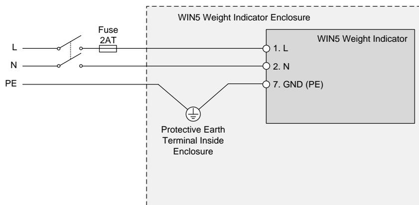
Figure 2.5 Connection of Power Supply and Protective Earth
