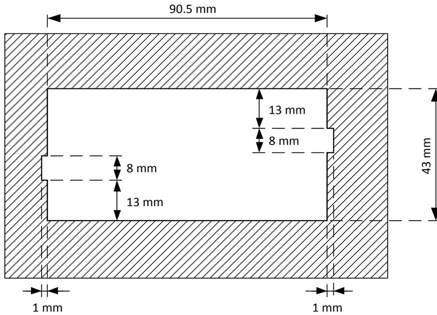
Figure 2.1 Recommended mounting hole dimensions
