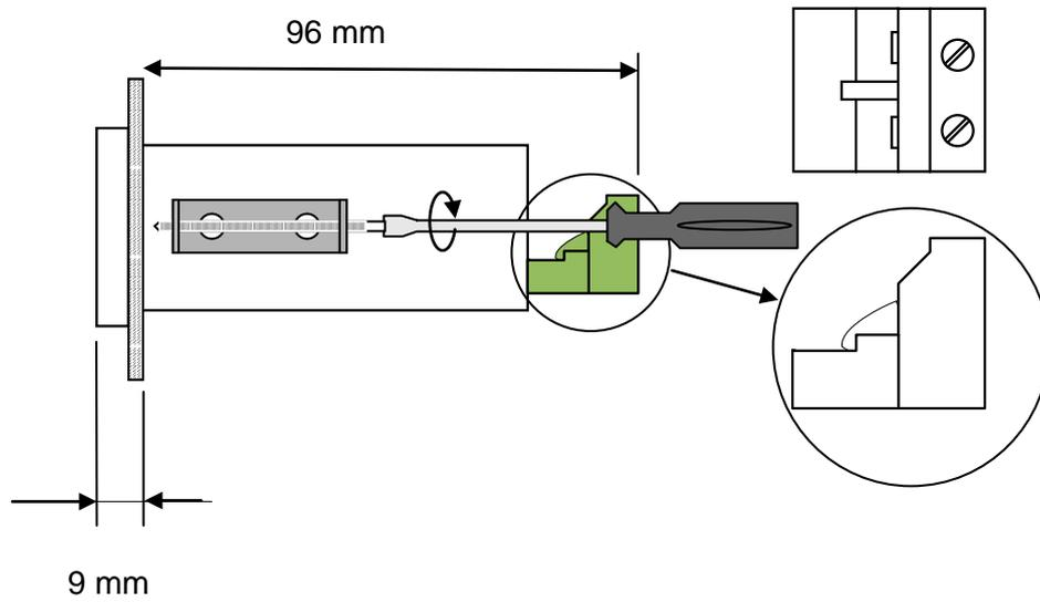
Figure 2.3 Installing of brackets, and dimensions.
