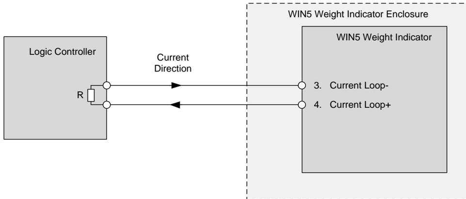
Figure 2.9 Connection of Current Loop Output
