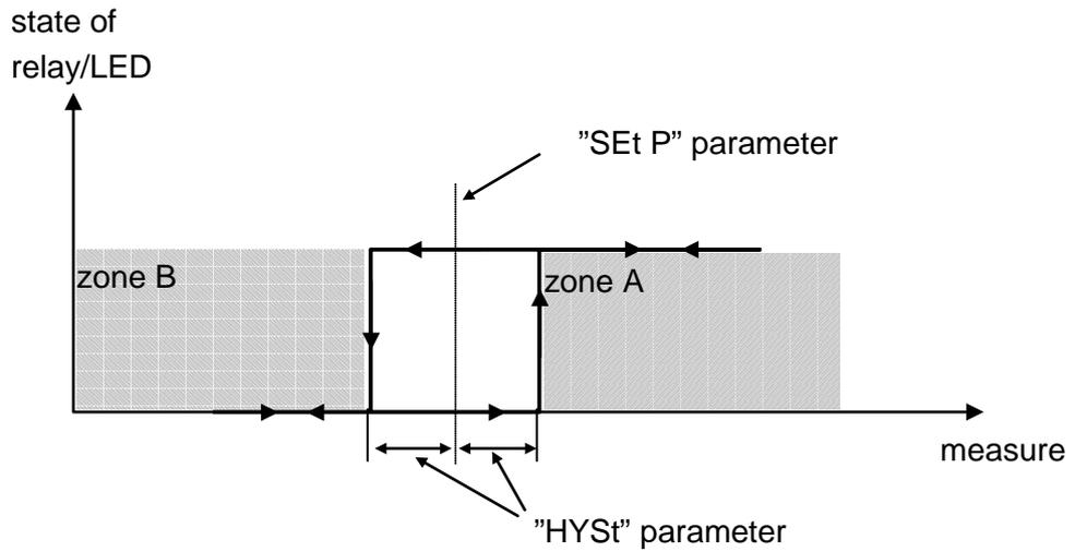
Figure 4.2 One threshold control of the relay/LED outputs
