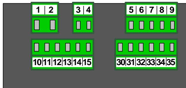
Figure 2.4 Instrument Screw Terminals at Rear Side
