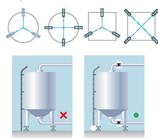
To achieve good weighing results, always use flexible connections to the vessel and check that no ladders or other arrangements connect the weighed vessel to surrounding foundation, walls or roof.
