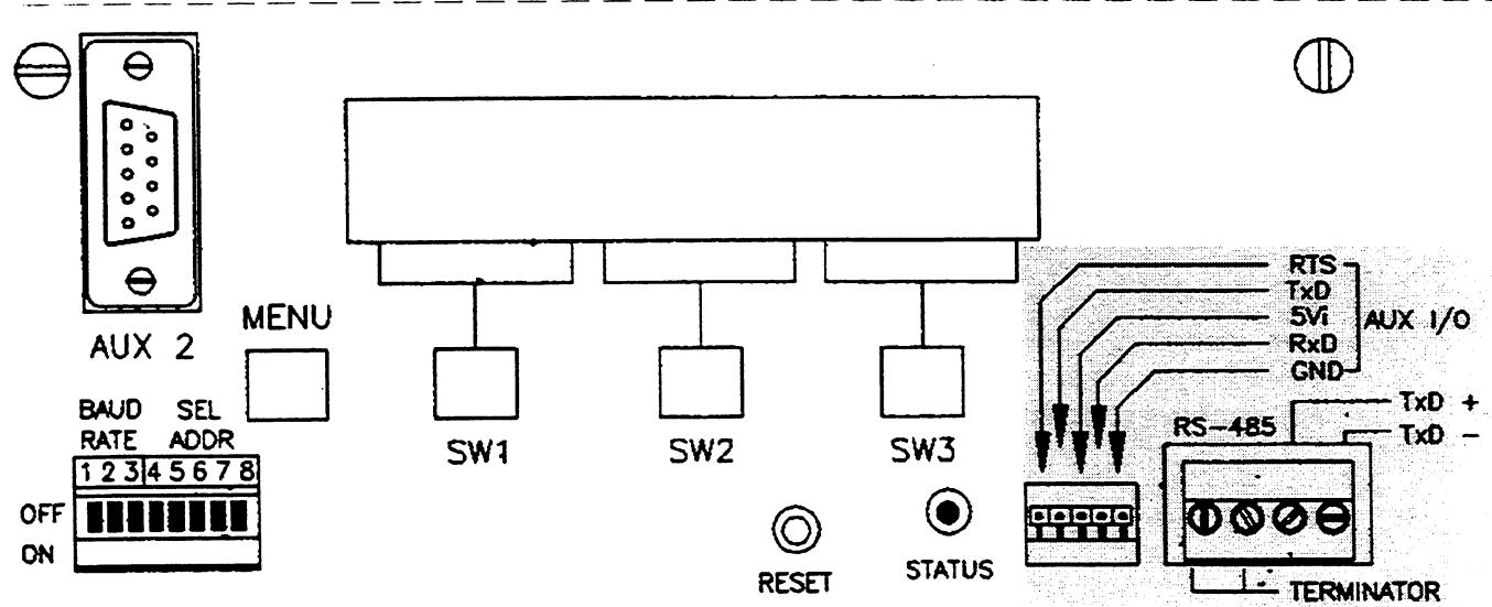
Figure 2-3. Serial Output Connections Connections (Shaded)
