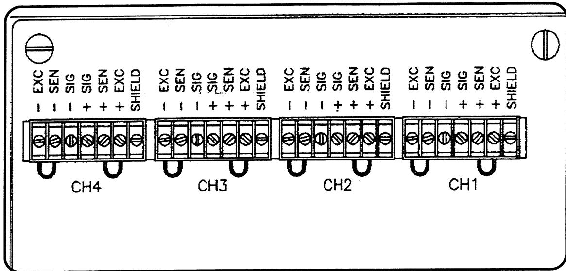
Figure 2-2. Load Cell Connections
