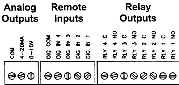
Figure 2-5. Optional I/O Connections
