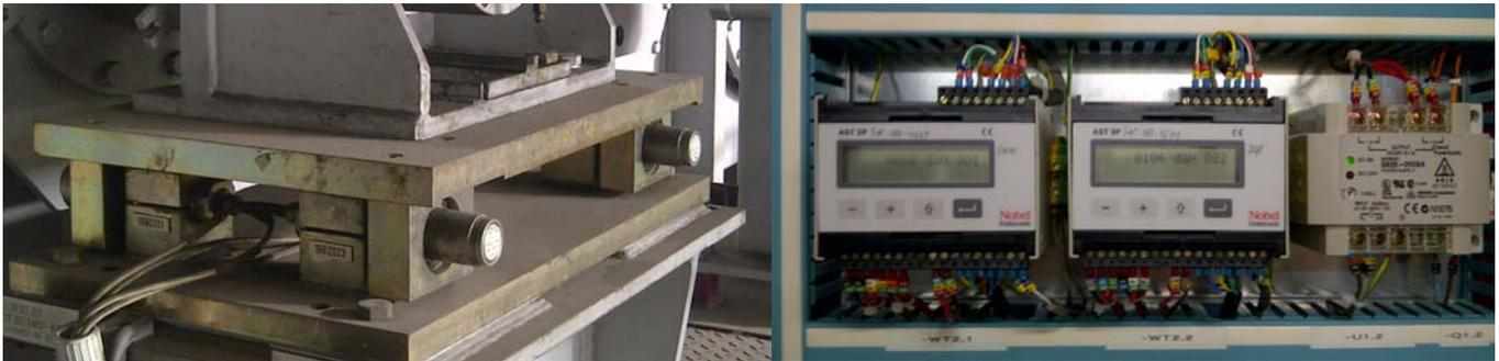
Figure 3: A PST web tension unit installed in a web tension measuring station, including the corresponding measuring amplifier
