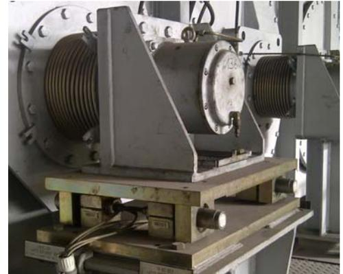
Figure 1: PST web tension measuring unit
