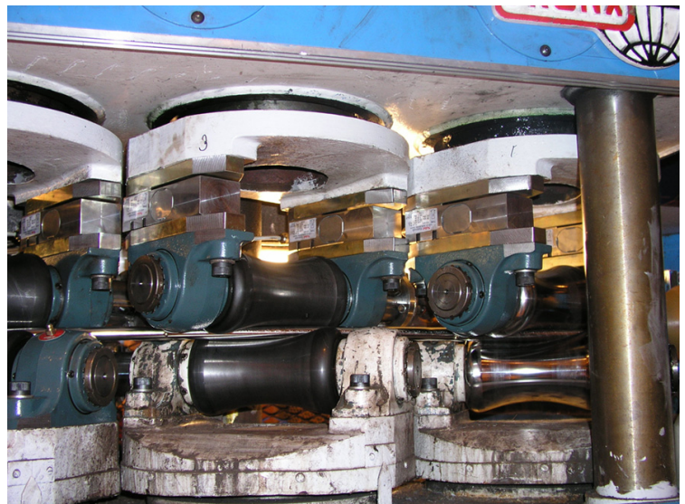
Figure 1: Rollers and KIP load cell in the strengthening machine
