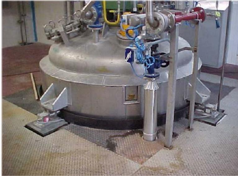
Figure 4: Heated tank with KIS-8 Load Cells
