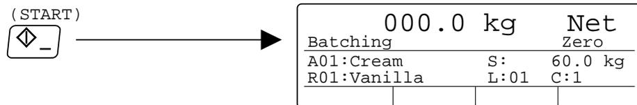
Batching can also be started from a digital input or via serial communication when normal weight is displayed, when menu Batching is open, and when the view Batching finished is displayed.
