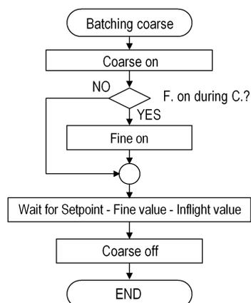
Figure 17. Flow chart for batching step "Batching coarse".
