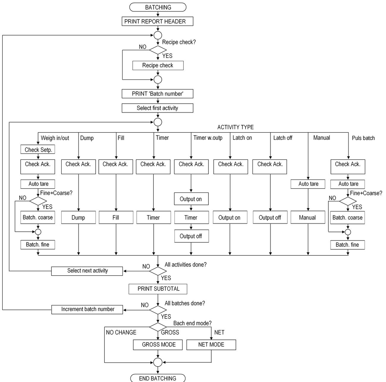
Figure 16. Principles for how batching is carried out. The batching sequence is a recipe that can include up to 30 activities. 30 such recipes can be stored in TAD 3.
