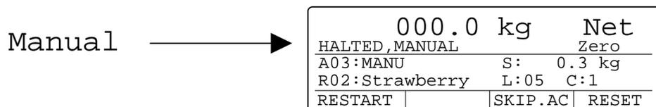
Alternatively the instrument can be set to allow manual entry by the digit keys of the added material weight value.
