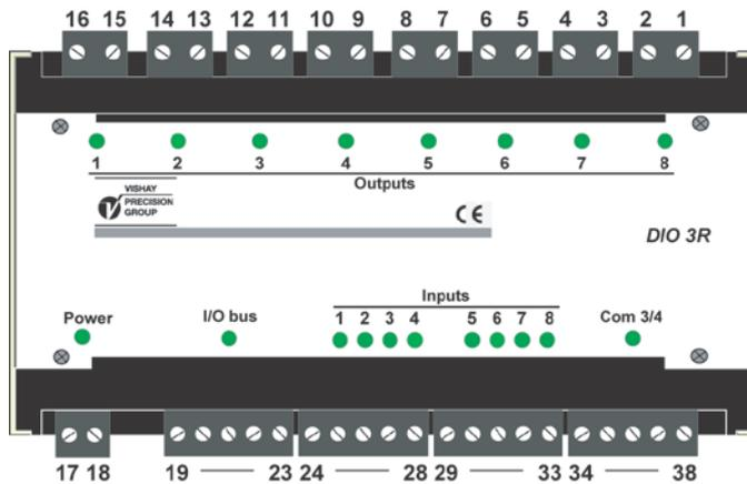
Figure 24. DIO 3R front panel and terminal blocks.
