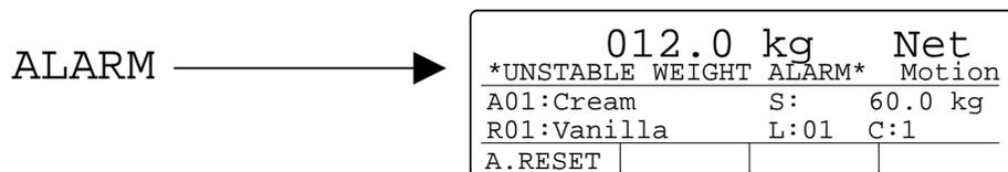
After the alarm has been reset, batching can be restarted, or it can be ended in different ways. See next page.
