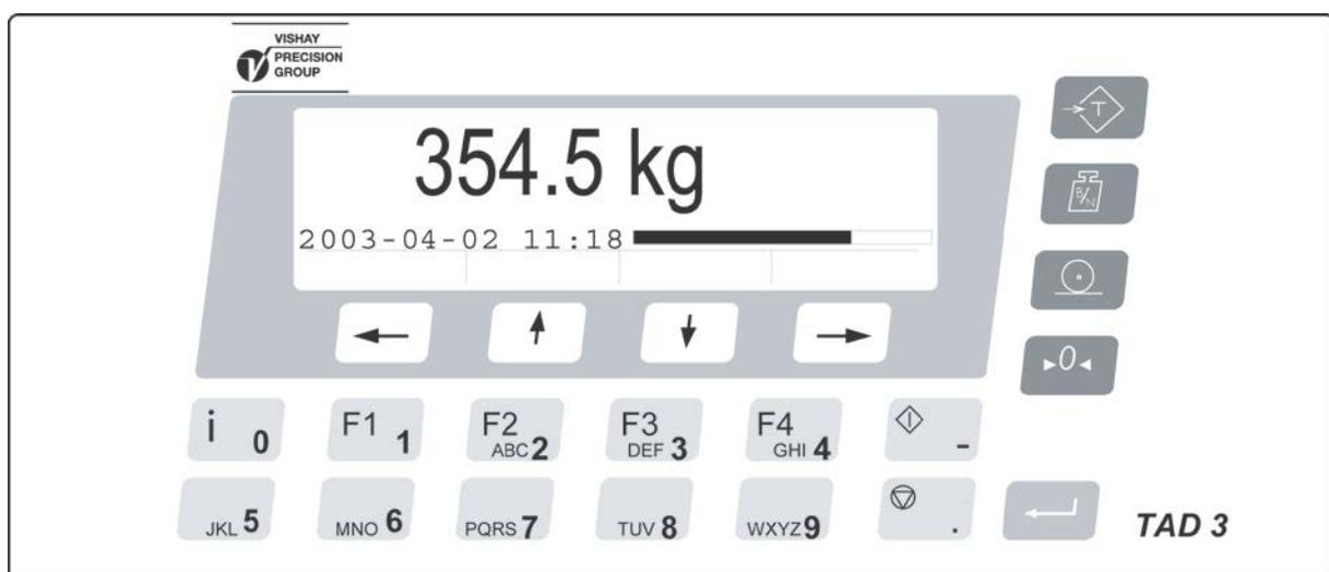
Figure 11. TAD 3 front panel by normal weighing operation.
