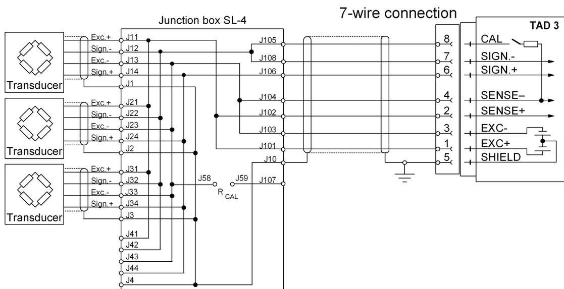
Figure 6. A transducer may be connected directly to terminals at TAD 3. For several transducers or long distance, a junction box and lengthening cable is needed.
