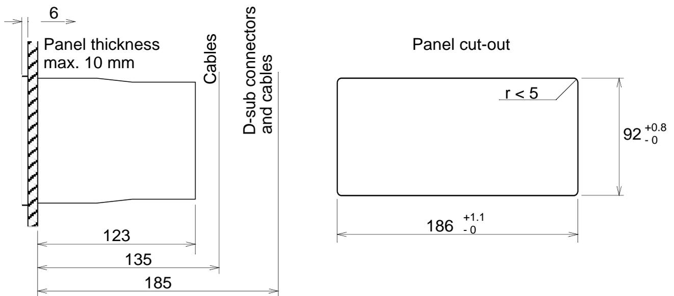
Figure 3. Mechanical dimensions and panel cut-out for TAD 3.
