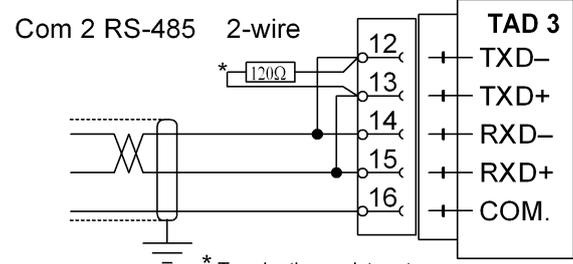
\* Terminating resistor at the last unit on the line.
