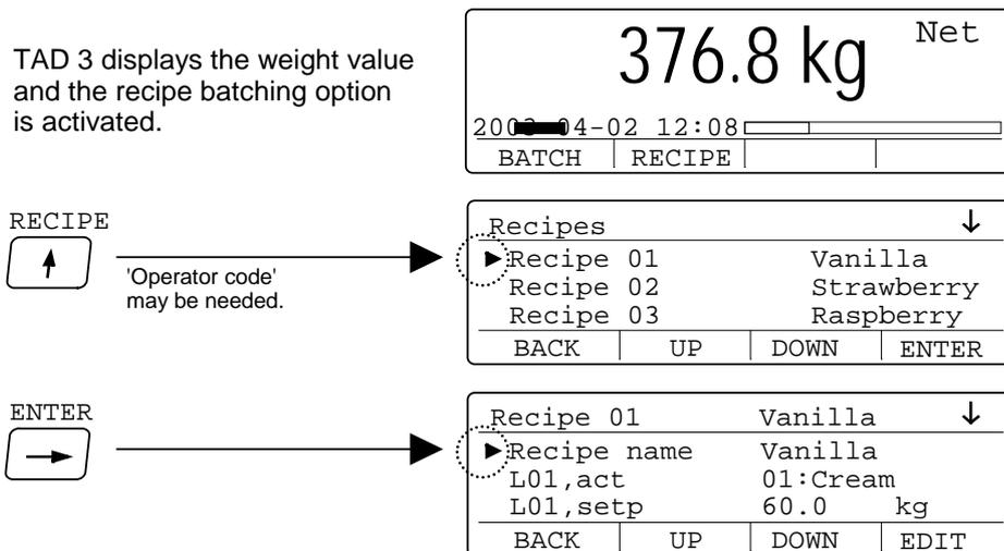
The Recipe menu displays a list of the 30 possible recipes. To the left is a cursor that can be positioned by function keys UP and DOWN.
