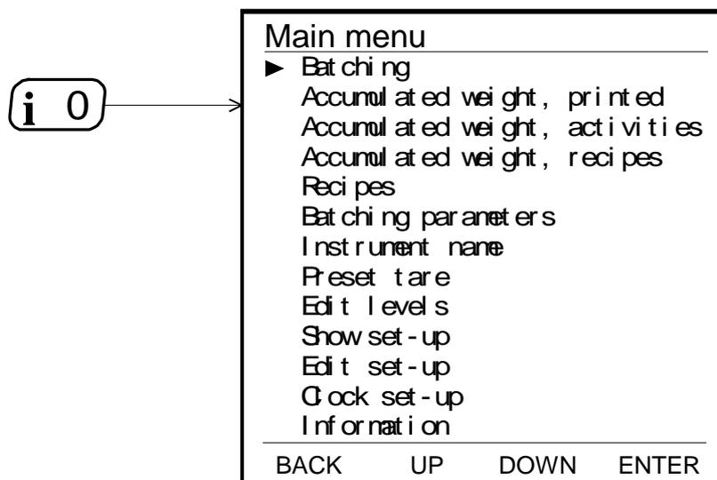
Figure 14. In the instrument Main menu a sub menu can be selected by the cursor and then opened by function key ENTER.
