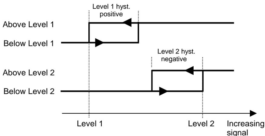
Figure 15. Influence on the level supervision from positive hysteresis, for Level 1, and negative hysteresis, for Level 2.
