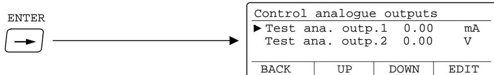
This menu can be opened, provided at least one of the parameters 'Output source' in menu Analogue outputs is set to something else than 'Not in use'.
