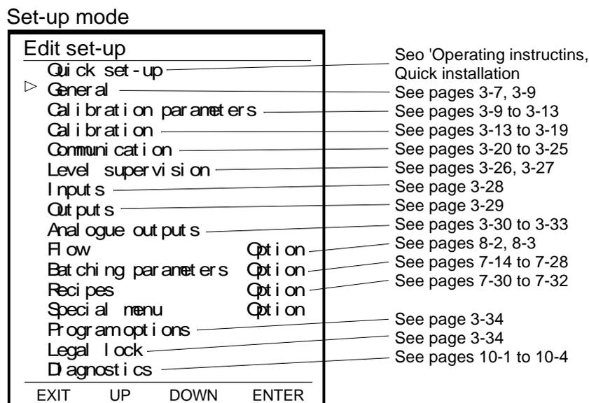
Figure 9. Menu 'Edit set-up' presents the names of the sub menus and has a cursor that can be positioned at any name.
