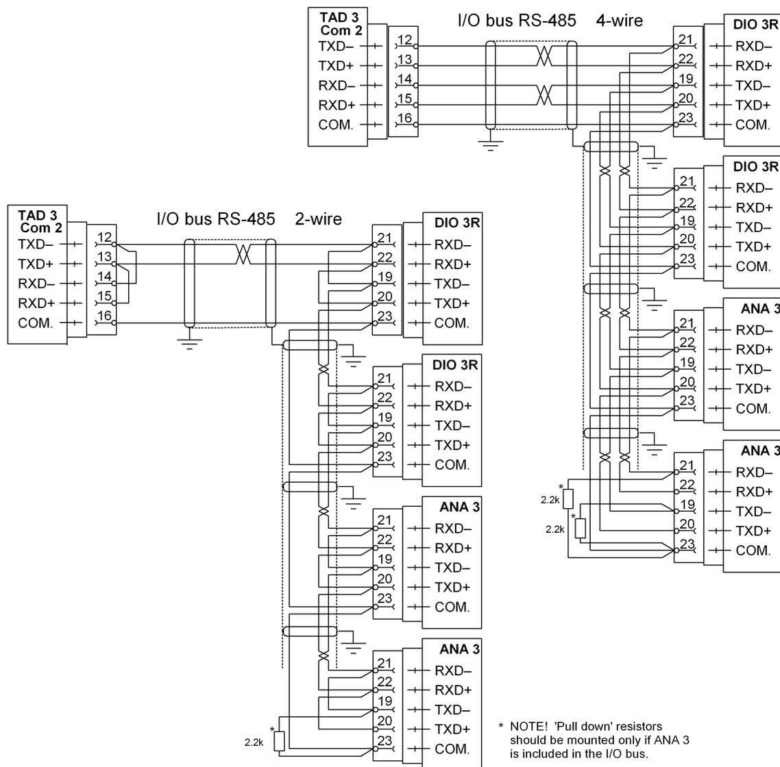
Figure 23. Examples on connection of two DIO 3R and two ANA 3 units to TAD 3 by 4-wire and 2-wire I/O bus cable.
