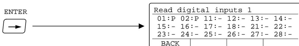
01 and 02 are internal inputs to TAD 3,
