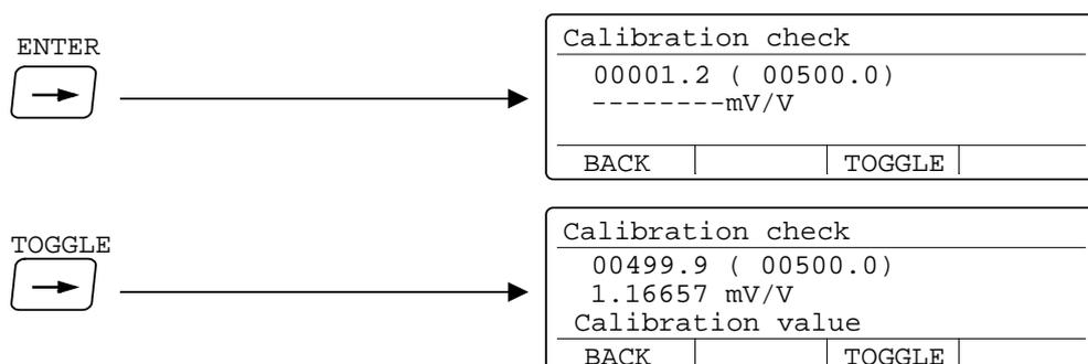
The menu 'Calibration check' is opened, showing actual gross weight and, in brackets, the scale capacity.
