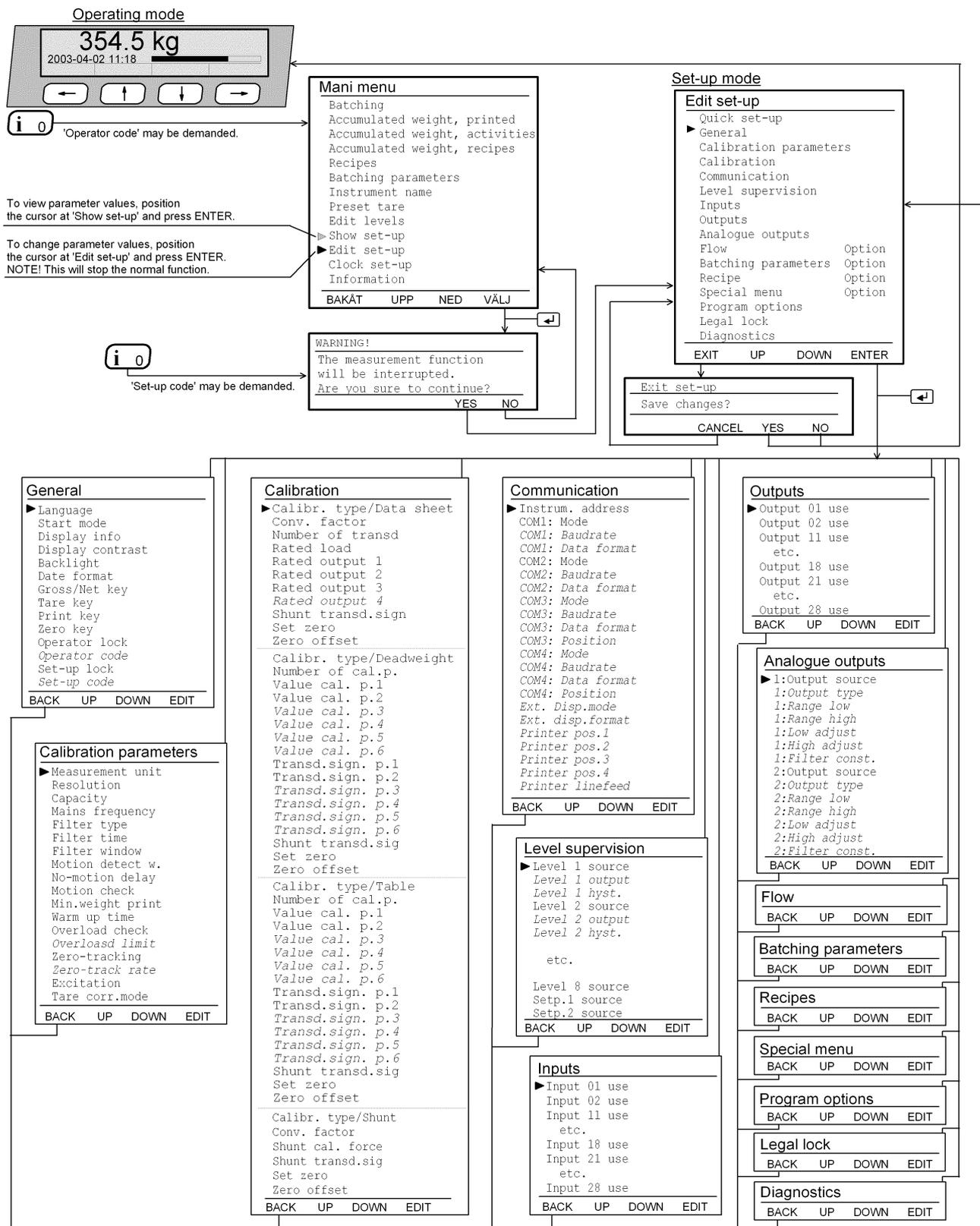
Figure 8. The parameters are arranged in a number of menus. For some parameters, viewing is conditional. Parameter editing can only be performed when the normal measuring operation is interrupted. Consequently, the selection of 'Edit set-up' must be acknowledged, and a valid code for a security lock may be demanded.
