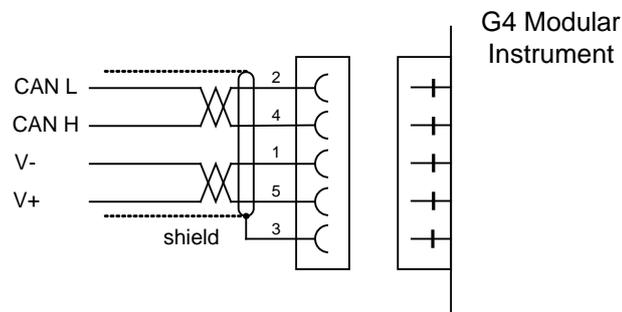
For reliable fieldbus function, line termination must be arranged in both ends of the transmission line. For a G4 Instrument placed at the end of the line, terminate line by placing a 121-ohm resistor between CAN L (pin 2) and CAN H (pin 4).
