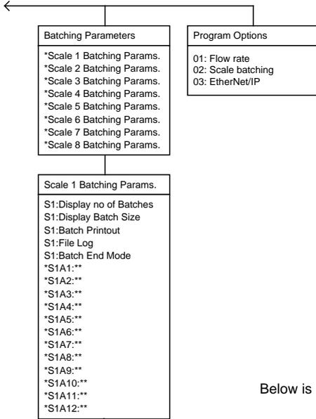
Below is shown the parameter set for each type of batching activity
