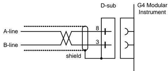
For reliable fieldbus function, line termination must be arranged in both ends of the transmission line. For a G4 instrument, at the end of the cable, a connector with line termination should be used. For all other G4 Instruments connection without line termination should be used.
