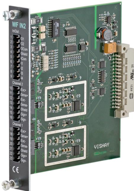
6-wire connection should be used if the integrated cable must be lengthened or if several transducers should be connected to one transducer input.
