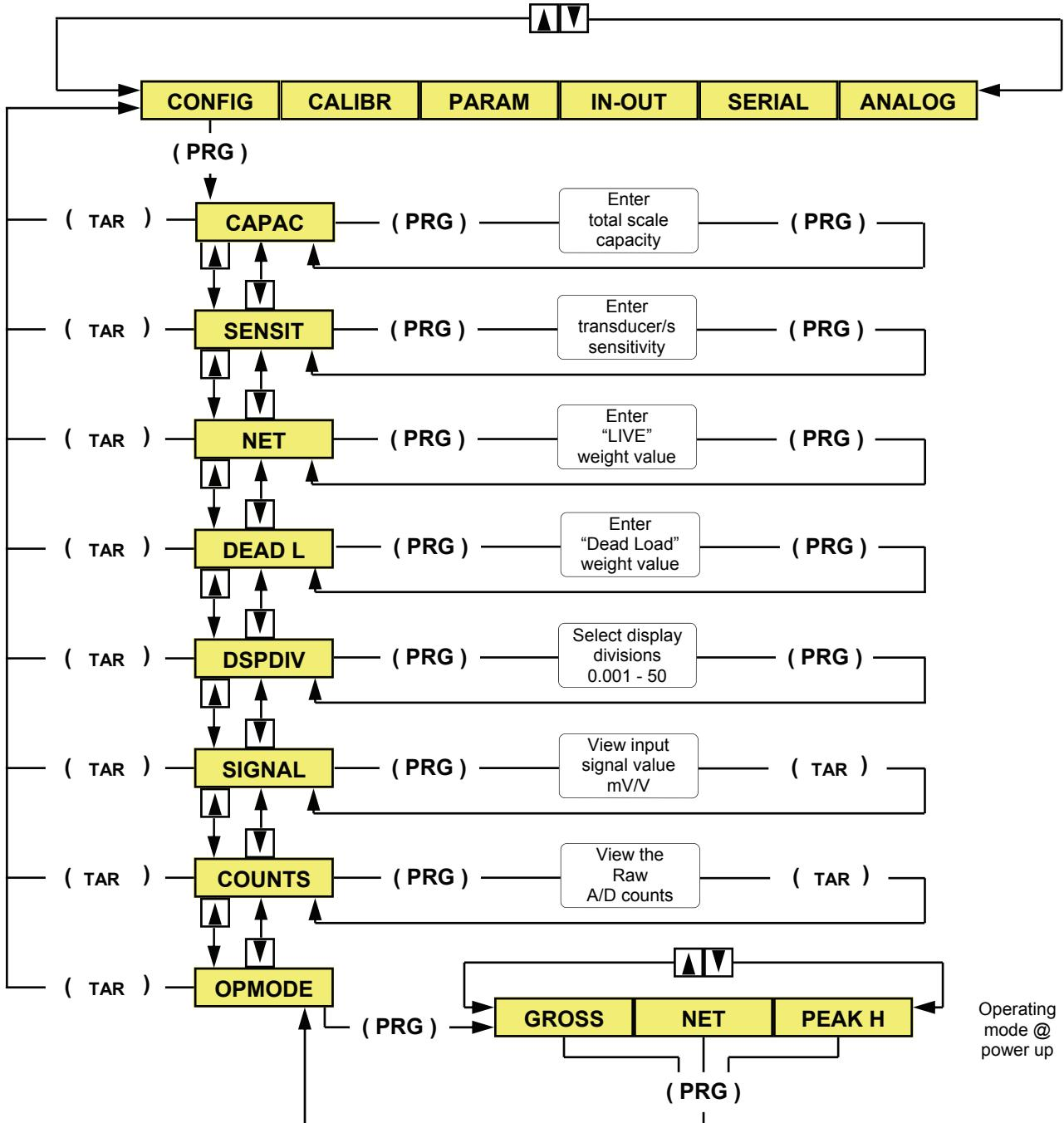
Place the unit in complete configuration mode by pressing and holding the "PRG" and "SET" keys on the front of the unit. The "SET" key must be pressed after the "PRG" key. Release both keys when CONFIG is displayed.
