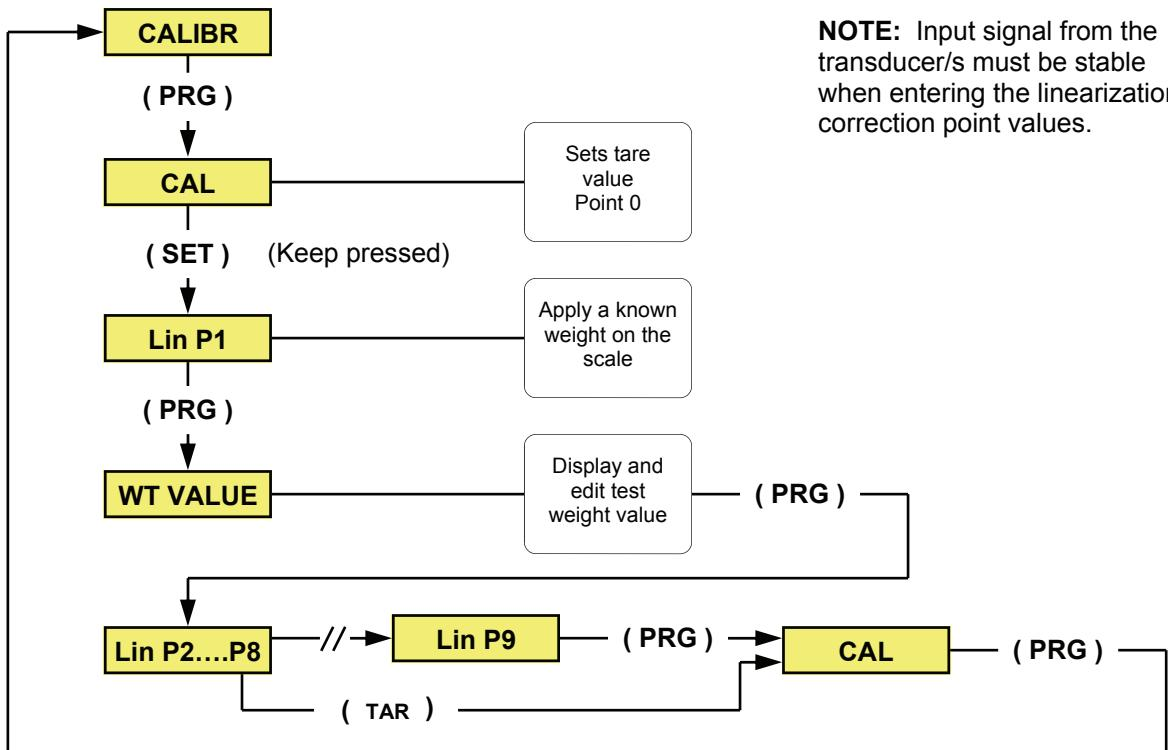
The Model PS-1045 features a 10-point linearization option (available only with the front panel keys). Any number of points up to 10 may be used, however, the last point *must always be* the full scale value of the weighing system.
