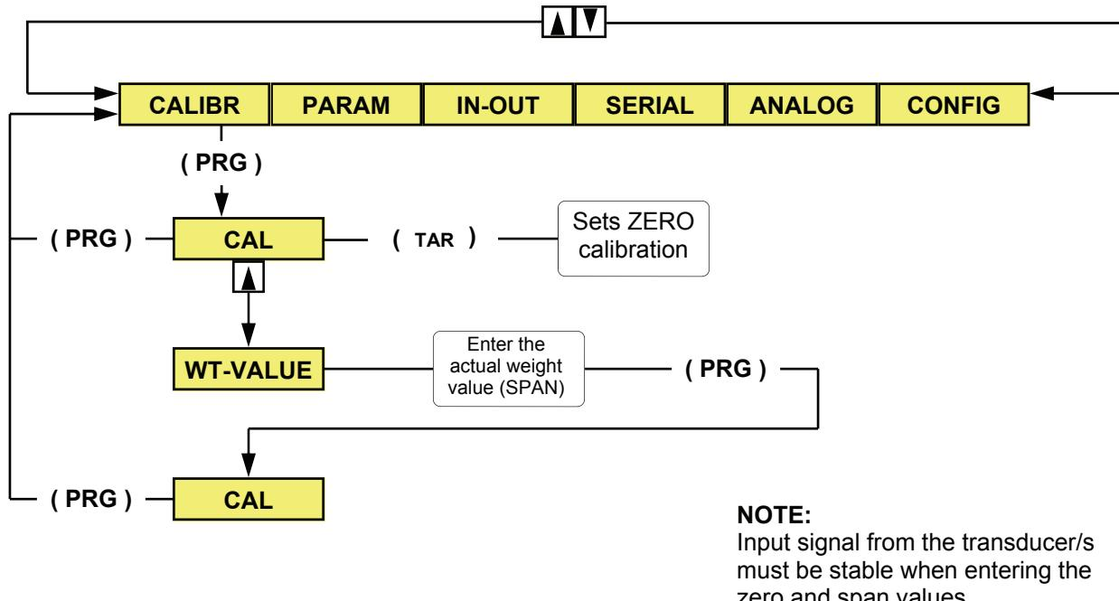
**NOTE:** Prior to calibration, the transmitter must be configured, thus giving it a set of operating parameters.
