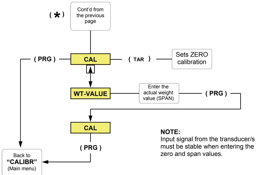
PS-1040 Series Transmitters can be calibrated via the front panel keys (PS-1045), or with the Pro-View configuration utility.
