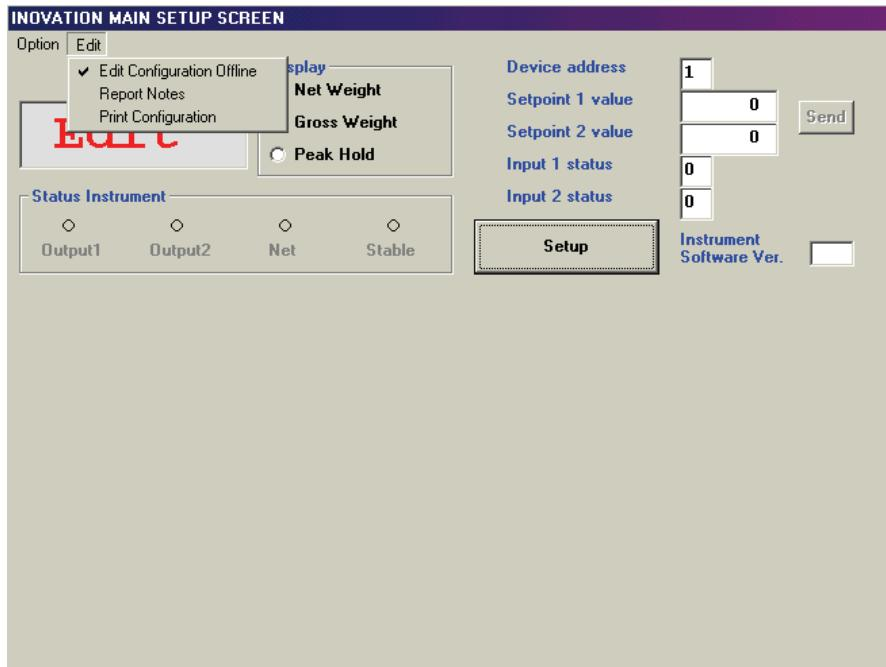
Starting from the 2.0 version, the Pro-View program allows the operator to create new configurations, save new files and open existing files **without having any instrument connected to the computer**.
