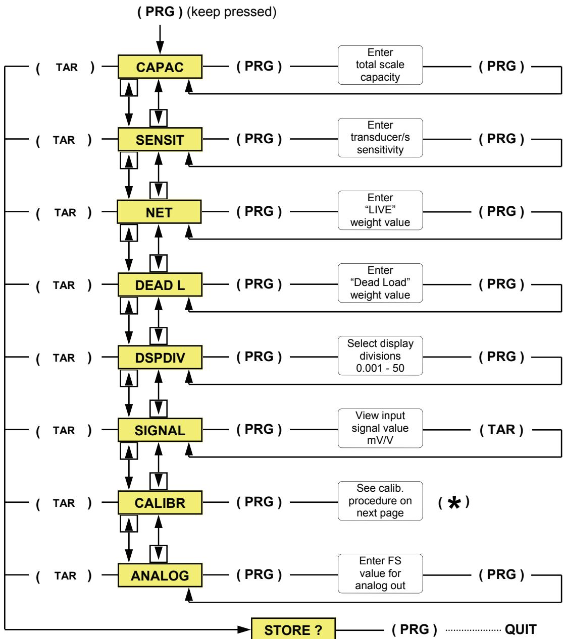
Place the unit in "Basic Configuration" mode by pressing and holding the "PRG" key until the display shows CAPAC. Use either the "UP" or "DOWN" keys to scroll through the eight basic configuration menus shown above. To set one of the following parameters, CAPAC, SENSIT, NET, DEAD L, DSPDIV, or ANALOG, press the "PRG" key to view the default or previously selected value for that parameter. To change the value, press the "TAR" key to select a digit,
