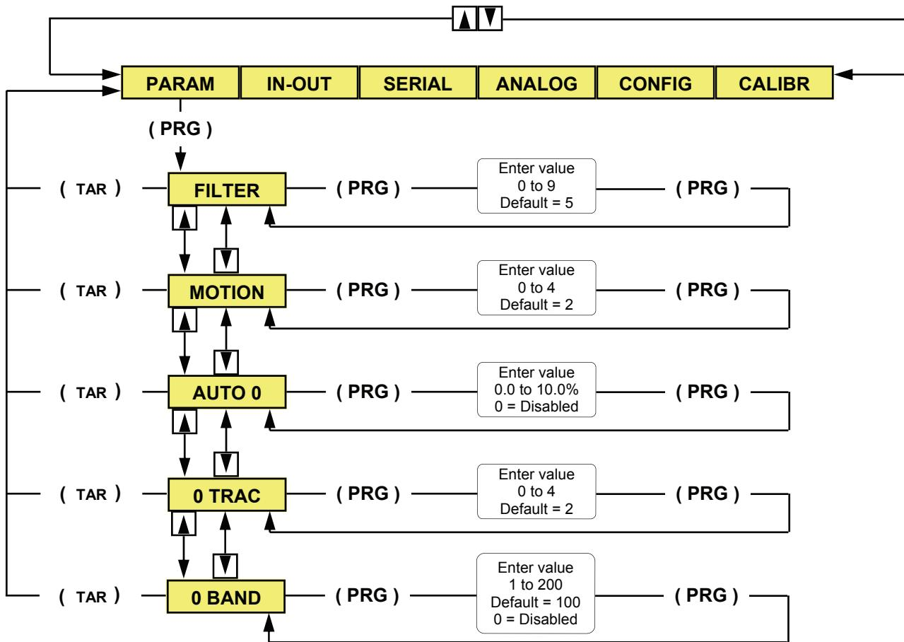
1. With the unit in "Complete Configuration" mode, press either the "UP" or "DOWN" keys until PARAM is shown on the display.
