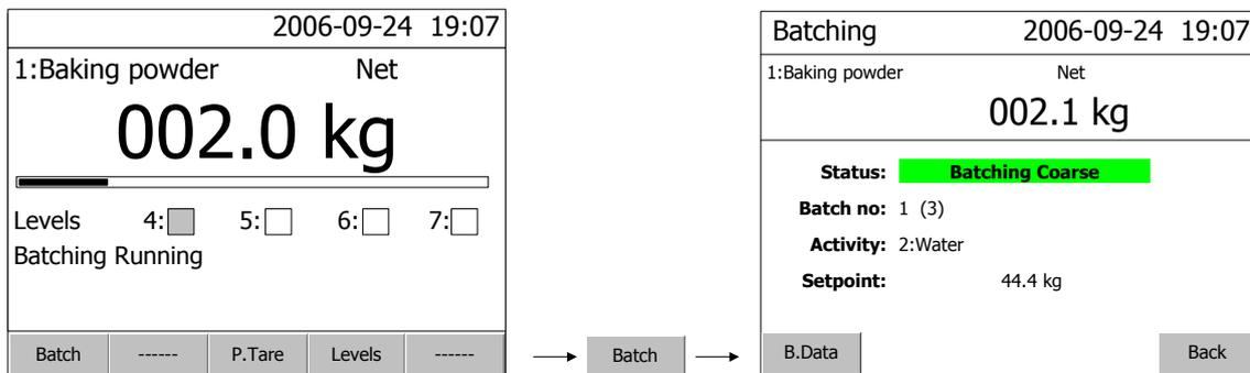
The batching display shows the actual weight and status for the selected scale. The display also shows all necessary information of the batching sequence that an operator needs to handle the batching process. Scales that are not batching will display status 'Inactive'.
