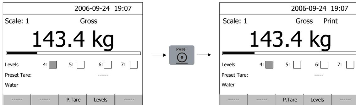
The print indication text 'Print' is shown where 'Zero' or 'Motion' indications normally appear. The print indication will appear even if no printer is configured and indicates that the weight is accumulated.
