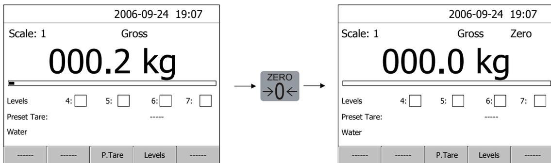
Zero adjustment can only be performed if the accumulated deviation from the basic zero setting in the last calibration is within -1 % to +3 % of the 'Capacity'. In other cases a new basic zero setting must be performed.
