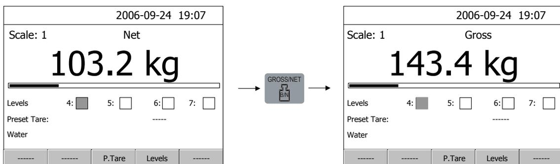
In some cases, gross weight is shown as a graphic bar at the display. Maximum length of the bar corresponds to 'Capacity' of the scale.
