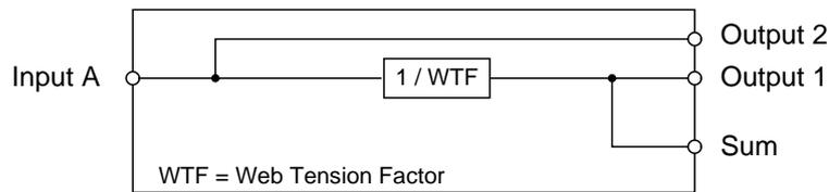
One Channel Function block, Web Tension mode
