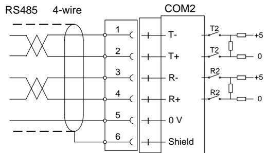
The communication lines must be terminated in both ends. If G4 is connected at the end of the communication line switches must be set as:
