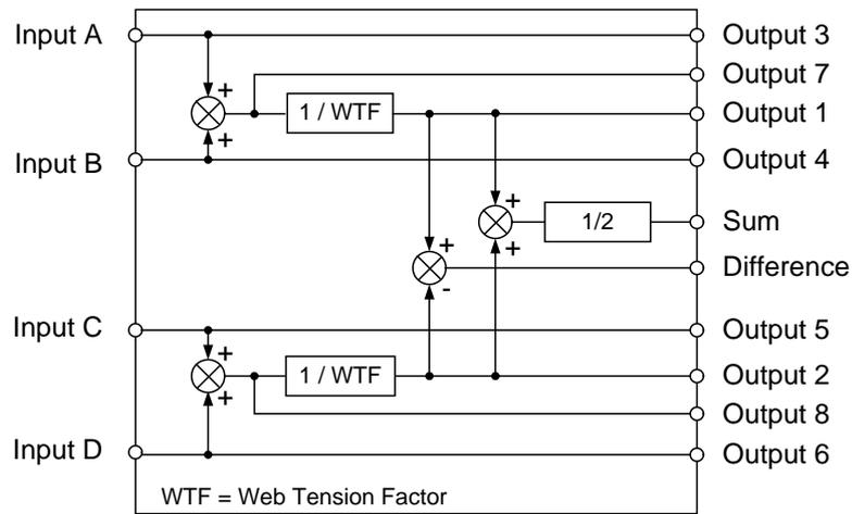
Four Channel Function block, Web Tension mode
