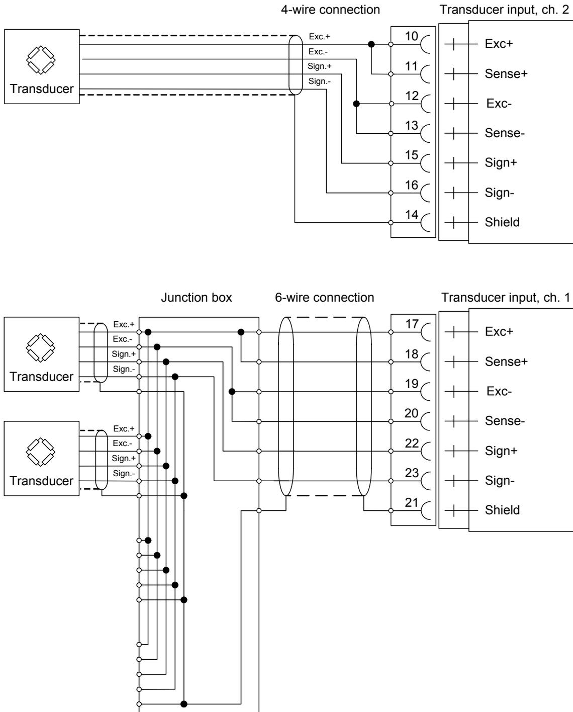
A transducer may be connected directly to terminals at the transducer input.
