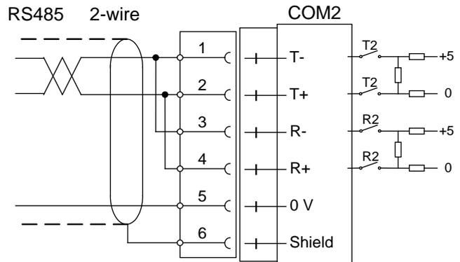
The communication lines must be terminated at both ends.
