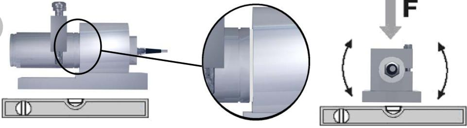
Level the LOAD MODULE within  $\pm 1^\circ$  in both directions. Control that the load cell silicone protection is aligned with bracket front (KIS-1-2-3-11).
