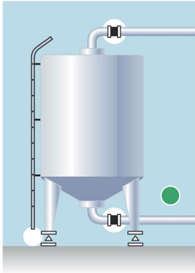
To achieve good weighing results, always use flexible connections to the vessel and check that no ladders or other arrangements connect the weighed vessel to surrounding foundation, walls or roof.
