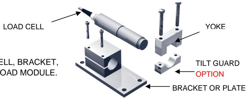
Assemble LOAD CELL, BRACKET, and YOKE to one LOAD MODULE.
