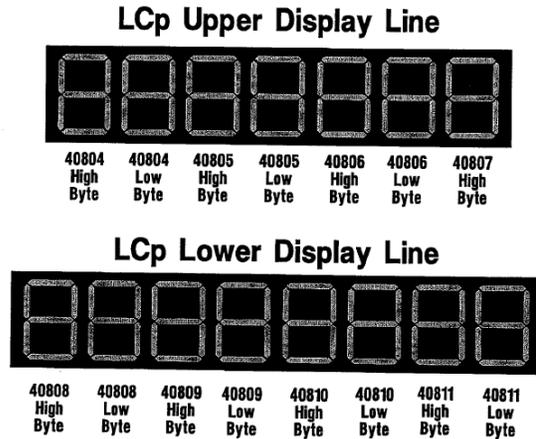
Figure 6-4. LCp-400 Front Panel Display Map.
