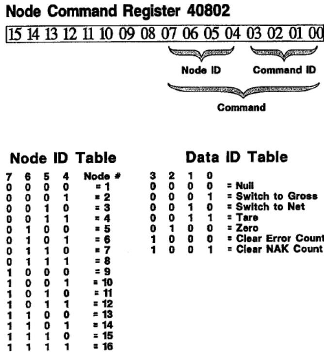
Figure 6-1. Node Command Register.
