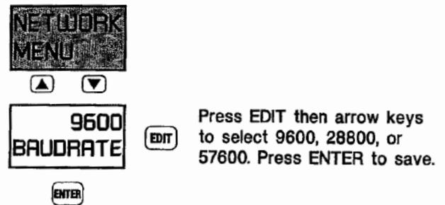
Figure 3-2. Network Baud Rate Selection.
