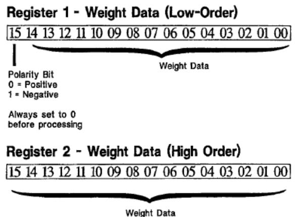
Figure 7-2. The Double Precision Word Format.
