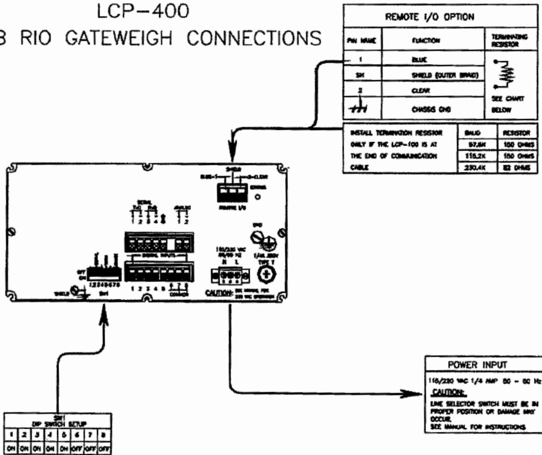
Figure 2-7. Remote I/O Wiring Diagram.
