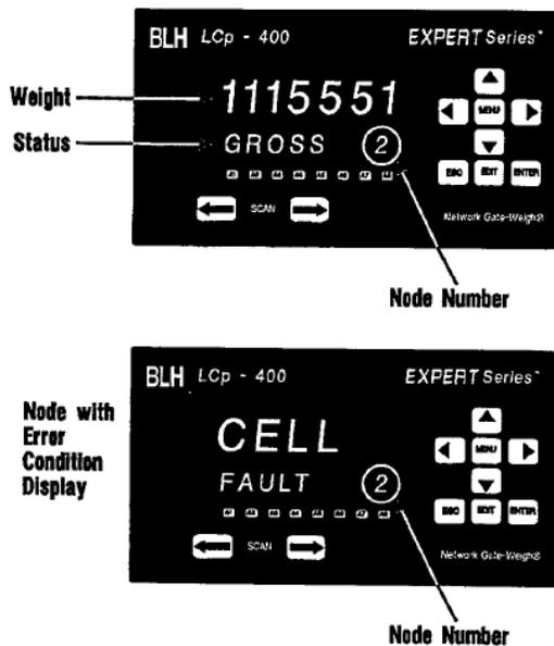
Figure 4-1. Node Display on LCp-400 Front Panel
