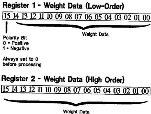
Figure 6-2. The Double Precision Word Format.
