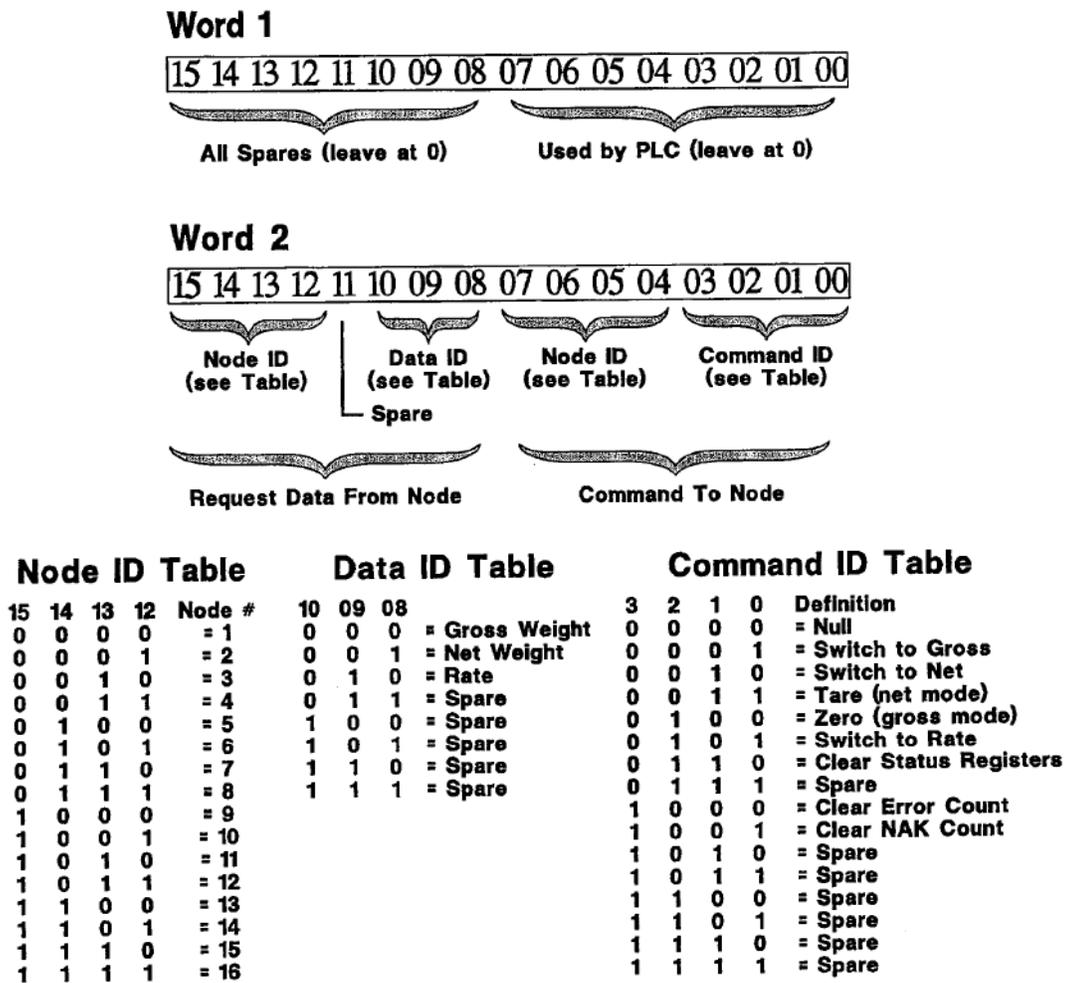
Figure 5-1. The LCp-400 Output Image Table.
