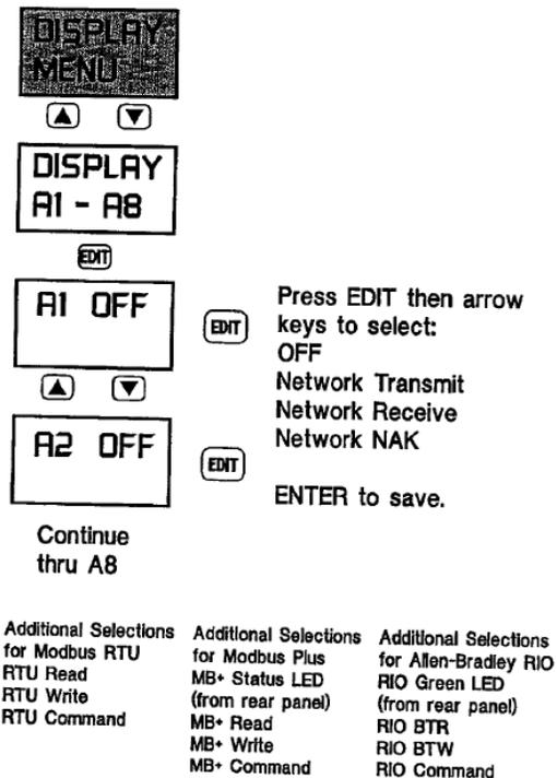
Figure 3-3. Display Annunciator Functions.
