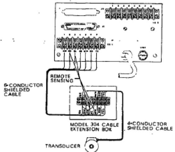
Figure 2-5, Remote Sensing Connections.
