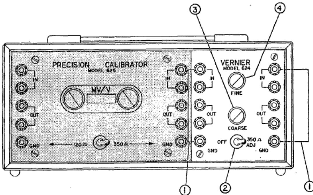
1. Color-coded Binding Posts. Right side posts are used for all interconnections with the equipment to be tested; left side posts are used for connecting the 624 with the 625.
