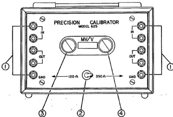
1. Attach the 5-conductor cable to the correct binding posts; 120Ω on the left side, 350Ω on the right side.
