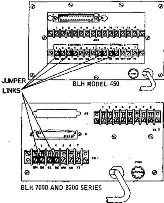
**Figure 2-6. Jumper Links Installed.**
