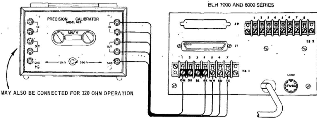
Figure 2-2. Typical Connections to Various BLH Equipment
