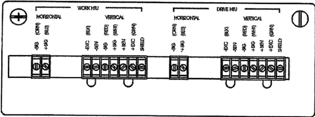
Figure 2-2. Load Cell Connections.
