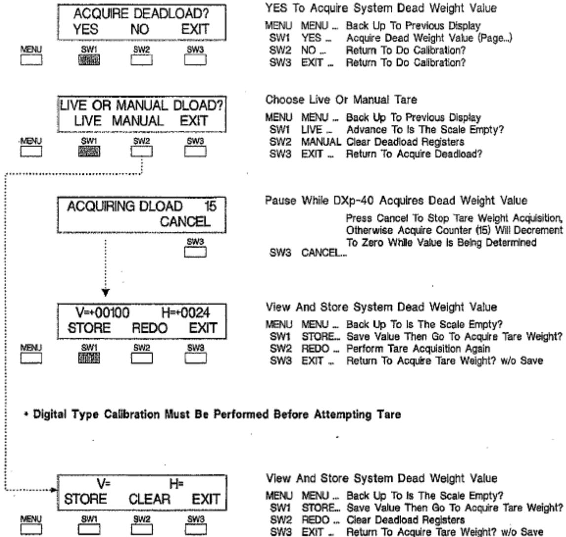
Figure 3-6. Acquire Deadload (Used with mV/V Cal Only).
