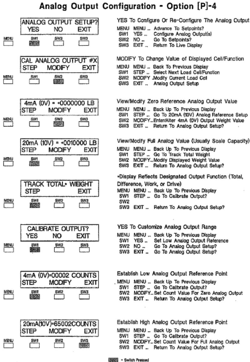
Figure 8-2b. Analog Output Configuration Flow Diagram.
