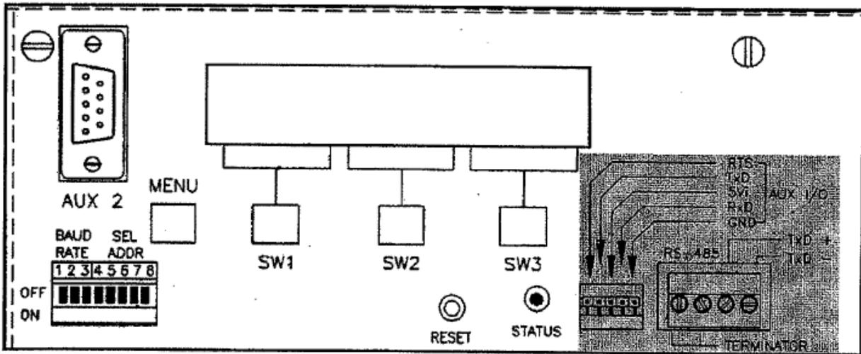
Figure 2-3 Serial Output Connections (Shaded).
