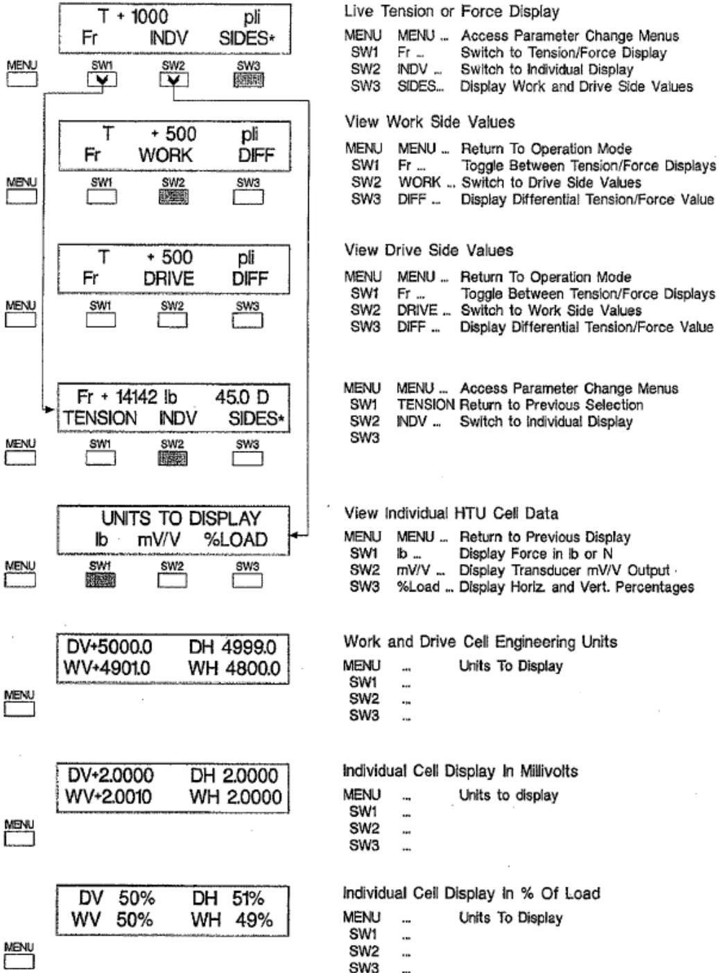
Figure 4-2. Switch Functions in the Operating Mode.
