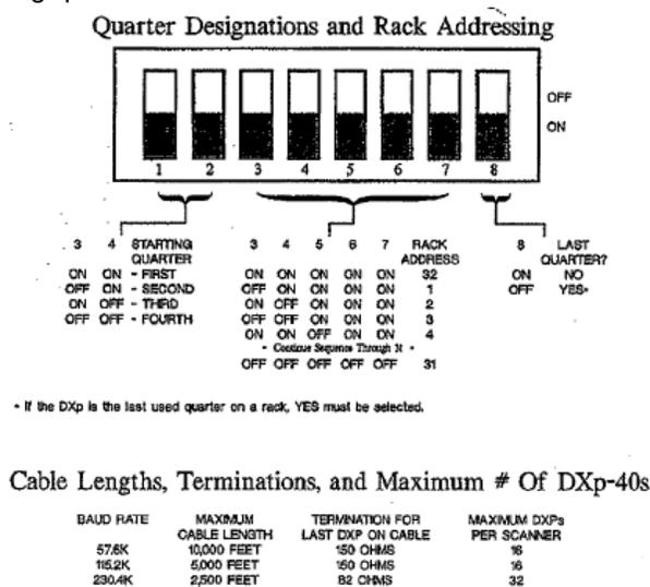
Figure 10-1. RIO Communication DIP Switch Settings.
