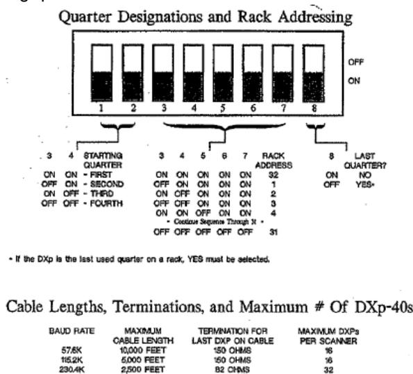
Figure 10-1. RIO Communication DIP Switch Settings.
