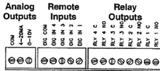
Figure 2-5a. I/O Connections for Process Options P-2, -3
