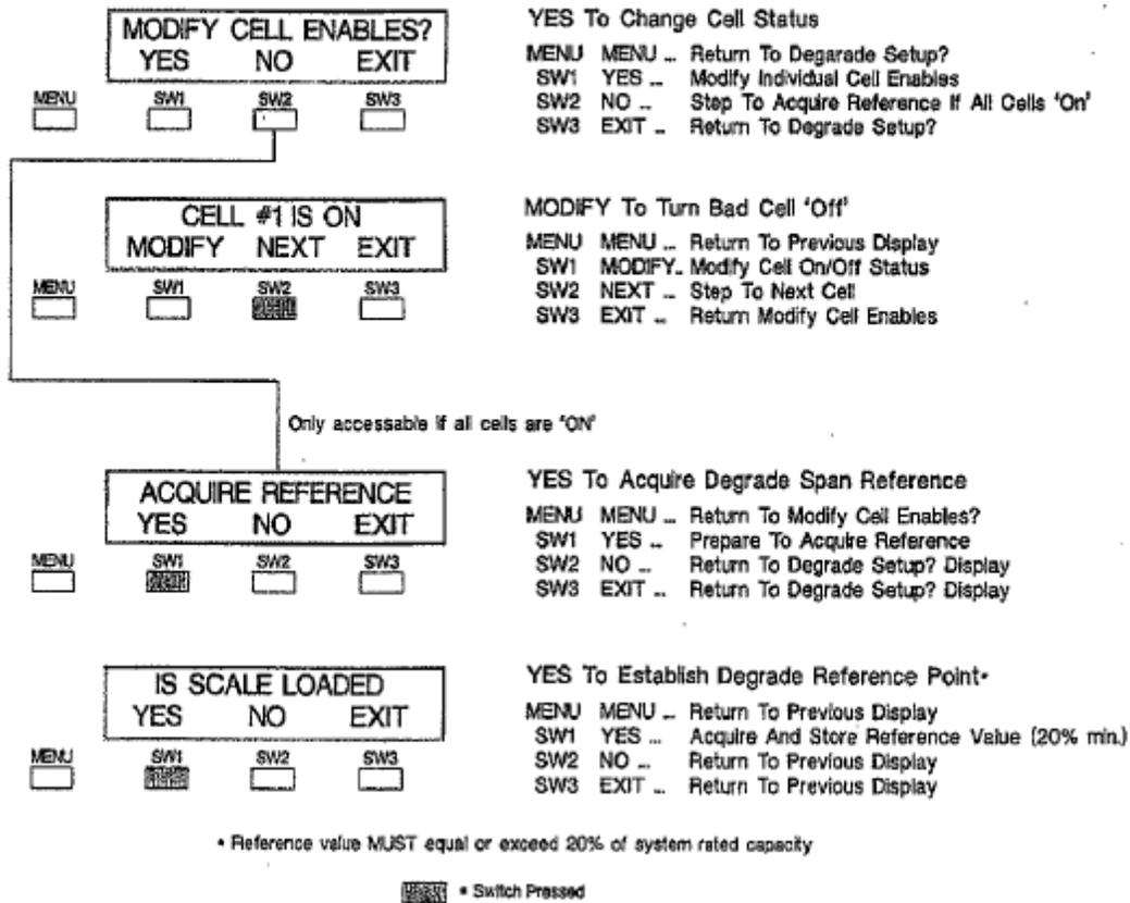
Figure 6-7. Degrade Mode Cell Selection and Reference.
