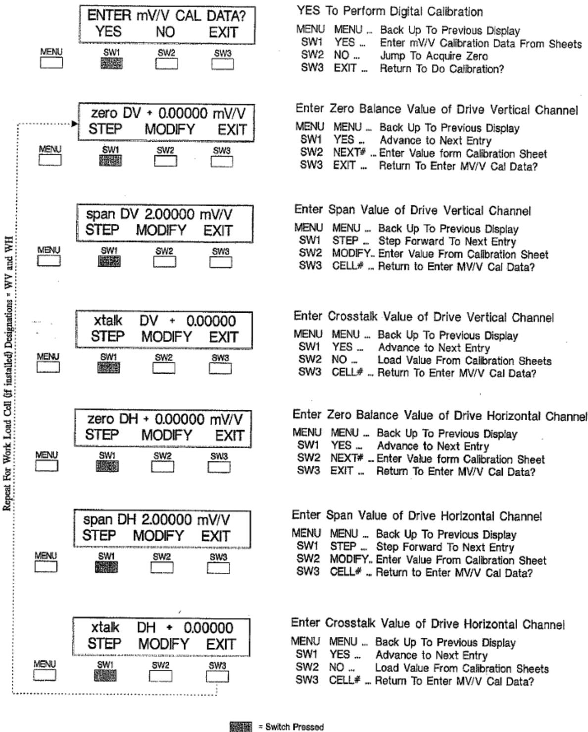
Figure 3-5. Millivolt per Volt Calibration Guide.
