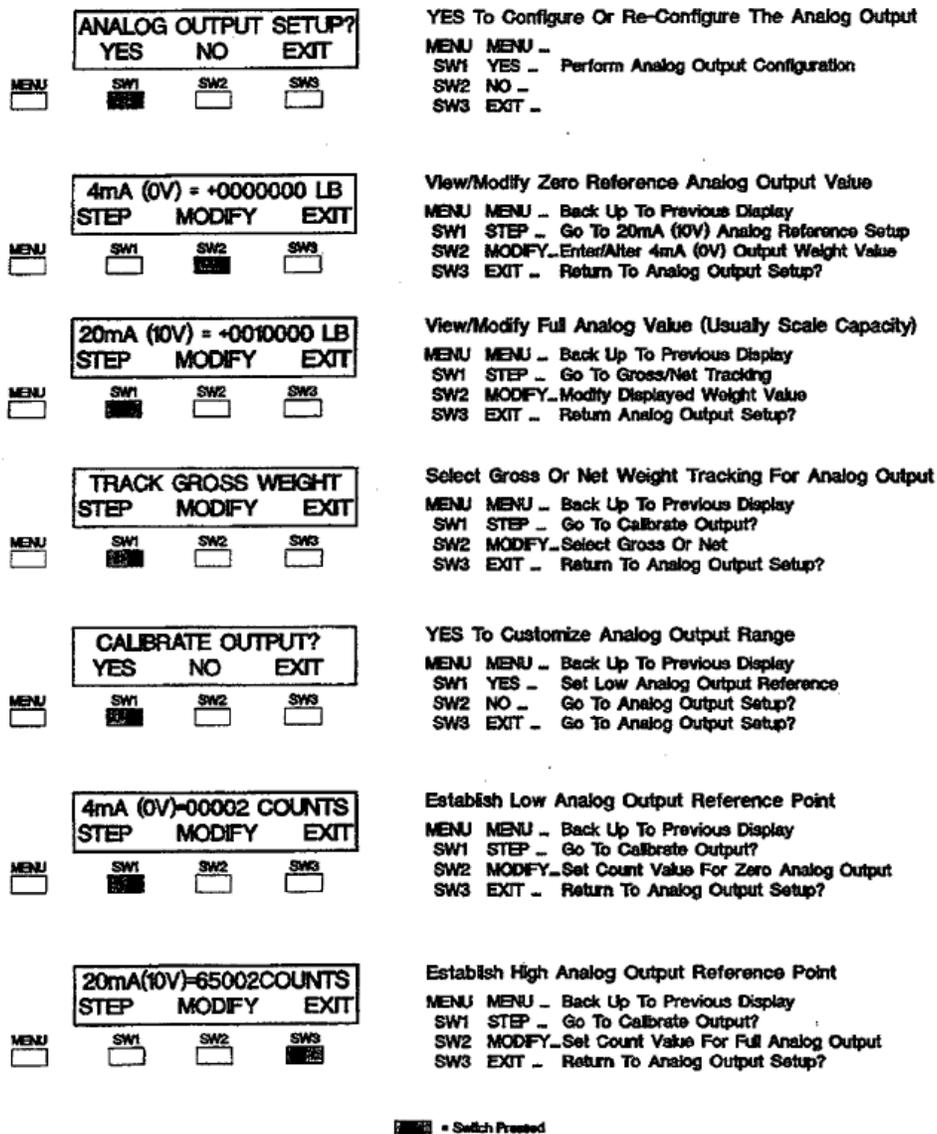
Figure 8-2. Analog Output Configuration Flow Diagram.
