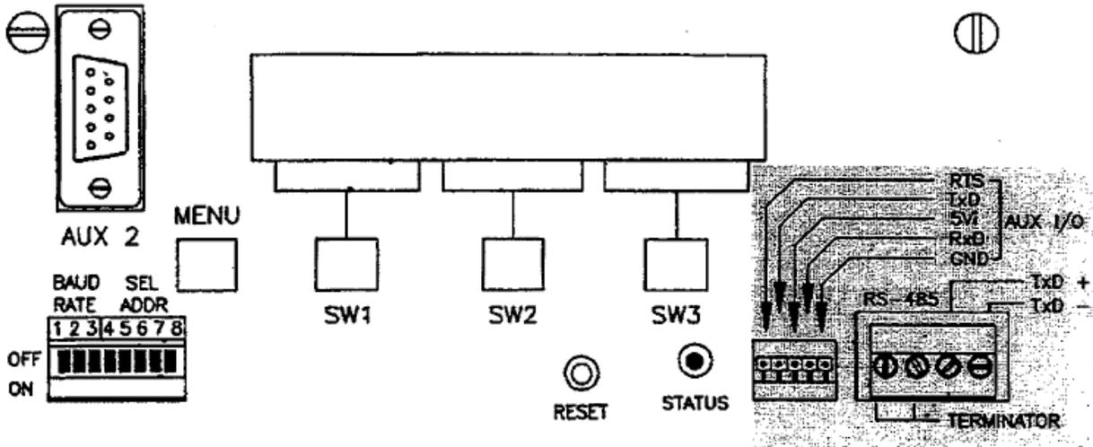
Figure 2-3. Serial Output Connections (Shaded).
