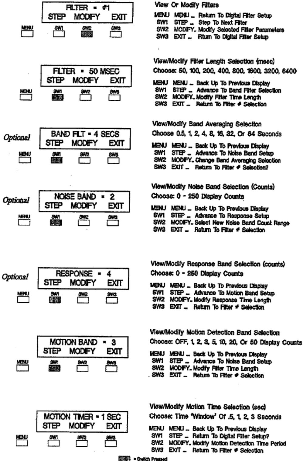
Figure 5-2. Digital Filter and Motion Setup.
