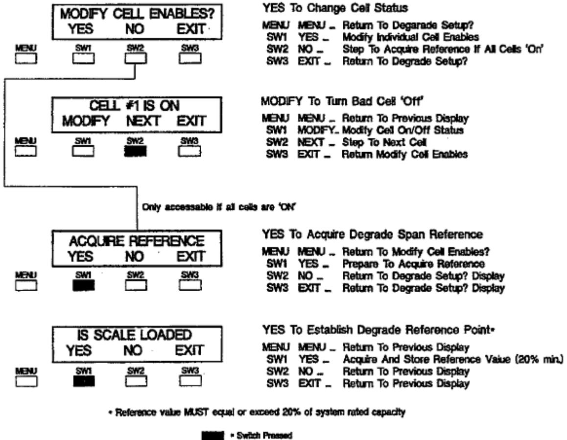
Figure 6-10. Degrade Mode Cell Selection and Reference.
