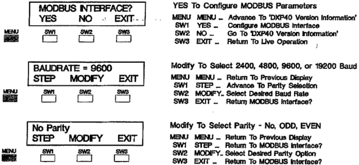
Figure 7-2. MODBUS Baud Rate and Parity Selections (accessed from main menu).
