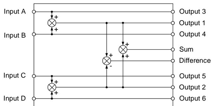
If input C is faulty the value is replaced by input D which means that input C and output 5 will have the same value as input D and output 6, and the value of output 2 will in fact be two times input D value.
