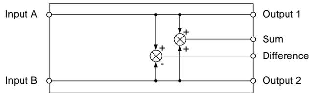
If input A is faulty the value is replaced by input B which means that input A and output 1 will have the same value as input B and output 2, and the value of output Sum will in fact be two times input B value (the value of output Difference will be 0).
