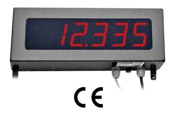
The RD10 is environmentally protected to IP65 and is suitable for outdoor use. A standard serial interface (RS-232 or RS-485 or 20 mA current loop) allows easy connection between the local indicator and the RD10 at distances up to 600 m (RS-485). The RD10 is fully compatible with BLH Nobel instruments AST 3P, WST 3, TAD3, G4 and G5.
