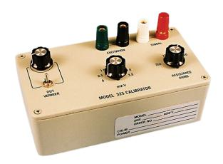
A built-in vernier adjustment provides a mV/V output signal from 0 to 106% of the selected range. Full range simulation tests setpoint cutoffs, auto-tare, auto-zero, overload, and other crucial instrument functions without loading the system.
