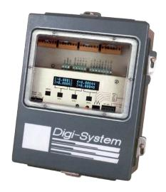
DXp-40 units provide designers with a wide range of communication and network options. Available "Easy Digital Interfaces" include Allen-Bradley Remote I/O, Modbus RTU, and conventional ASCII.
