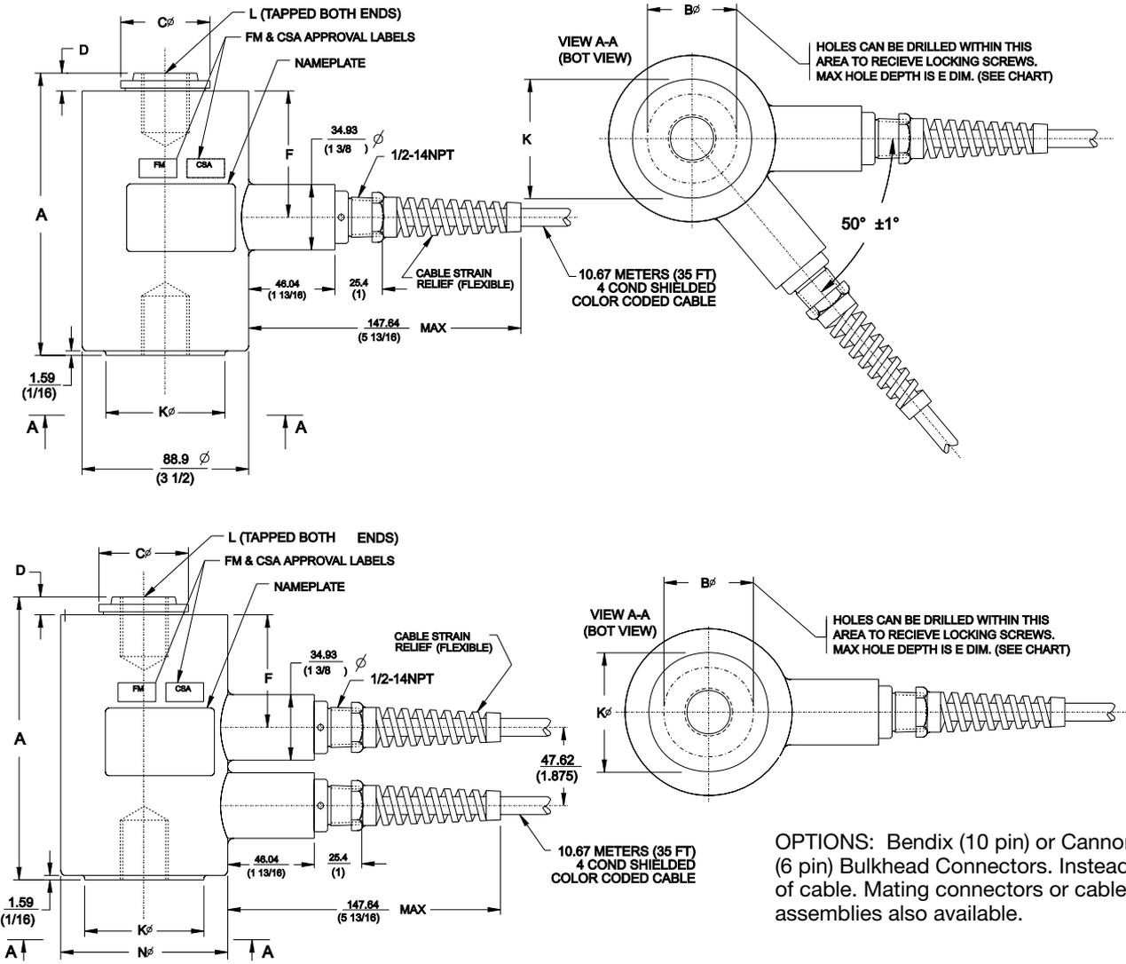
OPTIONS: Bendix (10 pin) or Cannon (6 pin) Bulkhead Connectors. Instead of cable. Mating connectors or cable assemblies also available.
