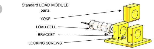
Check that there is a lateral play between YOKE and LOAD CELL by making sure that it is aligned with the LOAD CELL.
